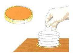
Using a template and a router, cut a circular hole in the surface of the Junckers 22 mm thickboard to allow the Frame to sit flush.
